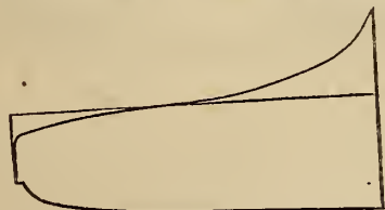
Low-pressure, bottom of cylinder, 42 in. diameter. Steam and vacuum as above.
